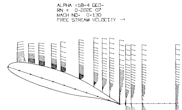
Fig. 4 Experimental velocity profile, \alpha = 18.4 deg.
